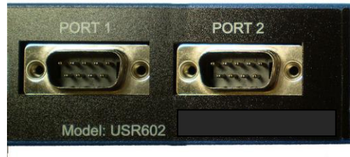
Figure 10: DB-9M Serial Port Connectors
