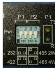
Figure 122: DIP Switches
